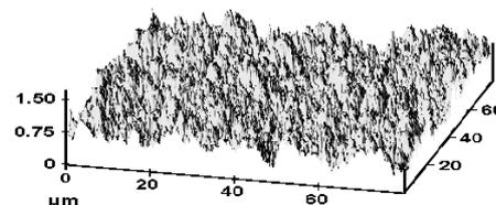
**Figure 1** Surface roughness measured over a 80x80 μm area by Atomic Force Microscopy (Source: Wake Forest University[5][6])
