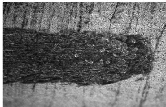
**Figure 10.** Wipe track on soft tin-plating with a contact radius 1.4 mm and normalforce 2 N after one pass.. The whole wipe track is plastically deformed. The track width is about 80  $\mu\text{m}$ .
