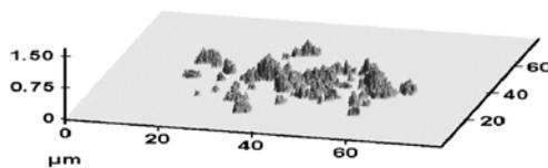
**Figure 3** The missing peaks from the surface of Figure 1 after impression with a ruby ball with  $0.8 \text{ mm}$  radius and  $1 \text{ N}$  force (Source: Wake Forest University)
