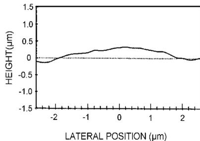
**Figure 2** One representative peak from figure 1 with equal horizontal and vertical scales (Source: Wake Forest University)
