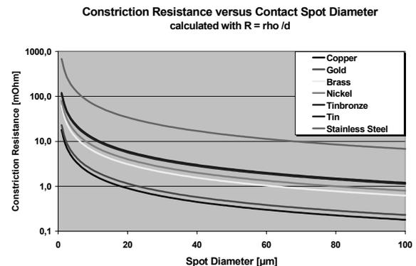
**Figure 5** The theoretical relation between constriction resistance and spot diameter for a single circular contact area with a clean and smooth metal surface for various metals (The lines from tin and from tinbronze coincide).
