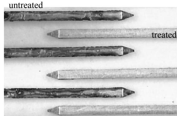
**Figure 13.** Untreated posts with a porous gold plating corrode heavily in a Flowing Mix Gas test, while posts from the same batch survive surprisingly well in the same test environment when treated with a conservating lubricant.
