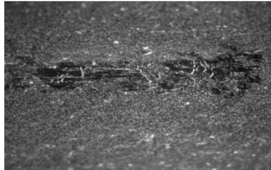
**Figure 9** Wipe track after one pass on gold-plating with a contact radius 1.4 mm and normalforce 2 N. Only the central part of the wipe track is locally plastically deformed, the track width is about 45  $\mu\text{m}$ .
