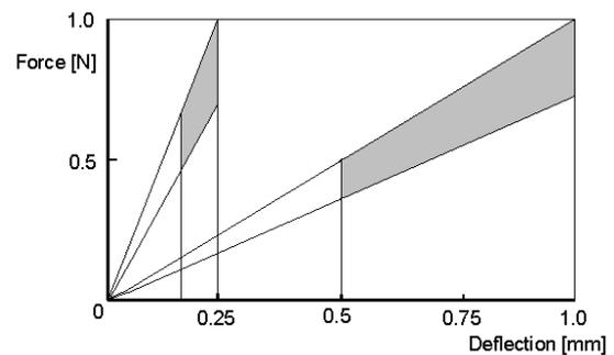
**Figure 7** Examples of two spring characteristics: the normal force depends on the spring deflection and on the spring rate and their respective tolerances.
