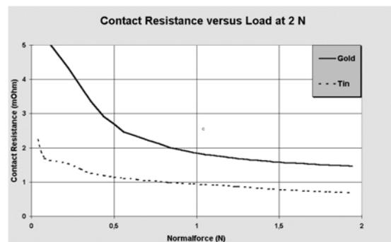
**Figure 11.** Contact Resistance versus Normalforce measurements during the loading phase of the gold and tinplated contacts from figures 9 and 10. Fresh tin is so soft that the contact resistance is lower and more stable than with gold, while the specific resistance of tin is much higher than that of gold.
