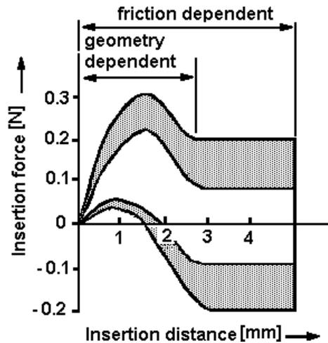
**Figure 9** The insertion force depends on the normal force, the contact geometry and on the co-efficient of friction
