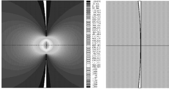
**Figure 6** The picture at the right shows a solid model of a contact surface. The black line at the surface is indicative for the thickness of a plating layer. The picture at the left shows the Hertzian elastic stress distribution around the same contact spot as calculated with the finite element method.
