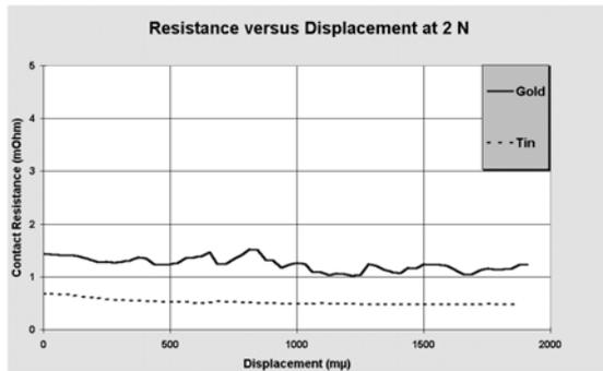
**Figure 12.** Contact Resistance versus Wipe Distance measurements during the wiping phase of the gold and tinplated contacts from figures 9 and 10. Fresh tin is so soft that the contact resistance is lower and more stable than with gold, while the specific resistance of tin is much higher than that of gold.
