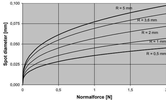
**Figure 4** Contact spot diameter according to Hertz theory versus normalforce for different values of the contact radius (sphere to flat).
