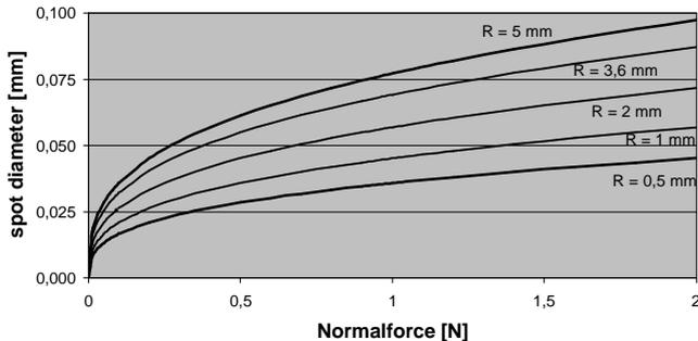
Fig. 3. Contact spot diameter according to the formula (2)
