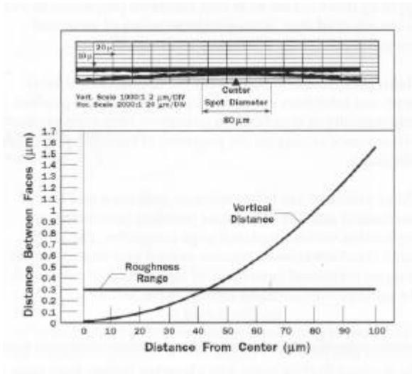
Fig. 5. Graph showing the measured roughness (top part) and the roughness range compared to the theoretical distance between undeformed surfaces (lower part)
