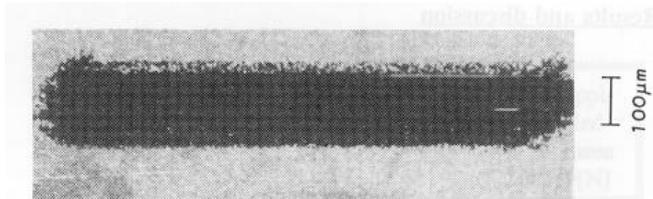
Fig.15 Wipe track for phosphorbronze, etched
