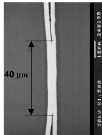
Fig. 9. SEM picture showing the cross-section of Fig. 8 at larger magnification with the gold (white) and the nickel layer (dark grey) near the contact point
