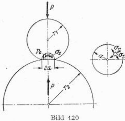
Fig. 1. Stress distribution between two spheres [7]
