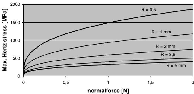
Fig. 2. Maximum Hertz stress as a function of normalforce, according to formula (1)
