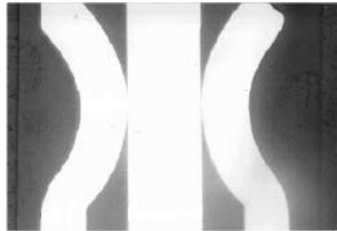
Fig. 8. Cross-section of pin and receptacle. The pin thickness is 0.4 mm, the receptacle material is 0.25 mm thick. The receptacle has a contact radius of 0.75 mm.
