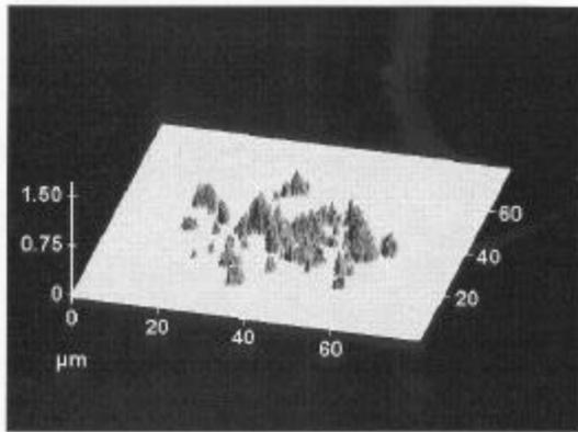
Fig. 13. The profile from Fig. 10 deduced from the undeformed profile, representing the changes due to the plastic deformation caused by the ruby ball [6]
