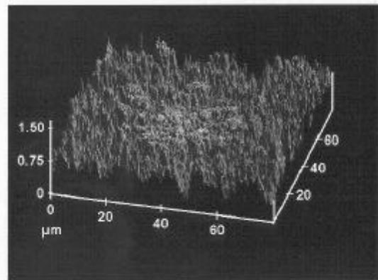
Fig. 11. Surface impression from a 1.6 mm ruby ball on a 1.25 μm gold layer over 1.25 nickel over a tinbronze (CuSn6) substrate. [6]
