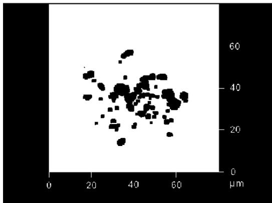
Fig. 14. Area plot, showing the projection onto the lateral plane of the difference picture of the change produced by indentation [6]
