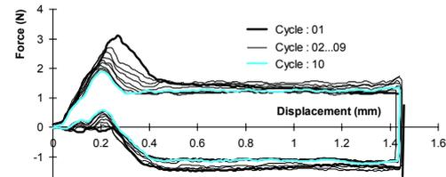
Fig 7. 'Without extra spring, lubricated', 10 insertion/withdrawal cycles.
