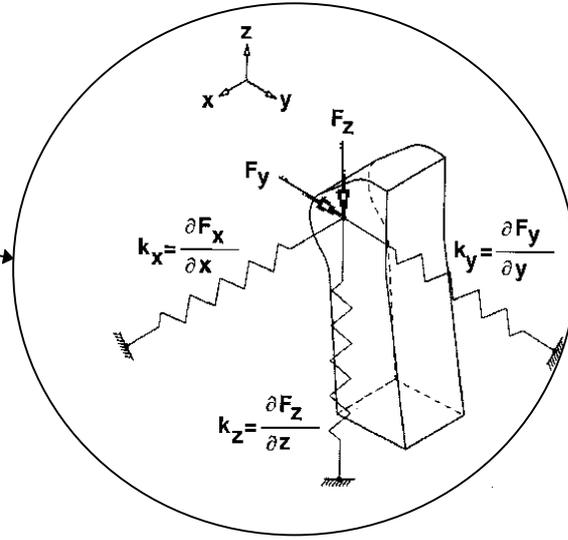
Figure 3. Scheme of contact region supported by springs
