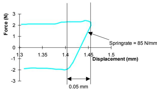
Figure 5. 'as received', transition from insertion to withdrawal.
