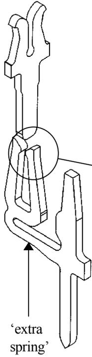
Figure 2. The Micro-MaTch™ contact system, with the extra spring arm.
