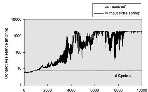
Fig 8. Contact resistance during 10,000 cycles.
