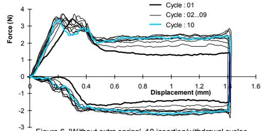
Figure 6. 'Without extra spring', 10 insertion/withdrawal cycles.
