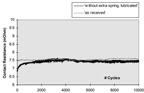
Fig 9. Contact resistance during 10.000 cycles
