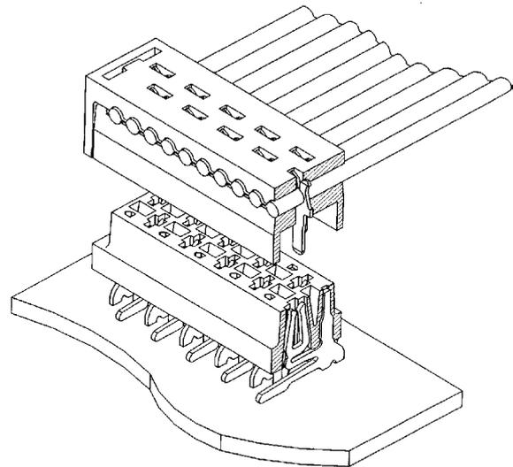
fig.1 The Micro-MaTch™ surface mount version connects a ribbon-cable to a PCB.
