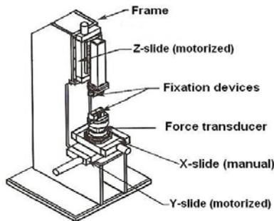
Fig.2. The DISC instrument, the tooling is mounted on the force transducer
