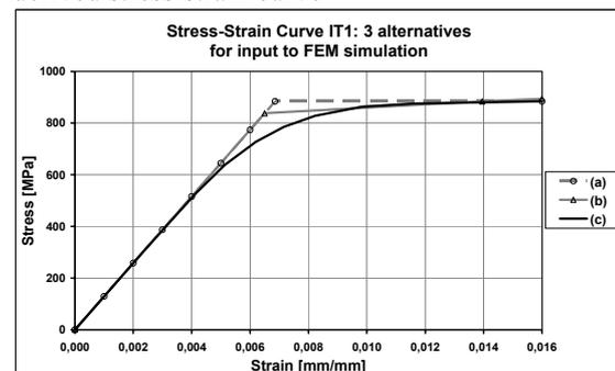
Fig. 12. Alternative FEM-inputs: curves (a), (b), and (c)
