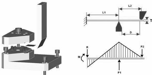
Fig.3. The measurement tool and mechanical scheme
