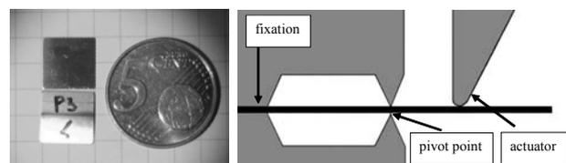
Fig. 1. A virgin and a tested sample compared with a 5 € coin in left picture and at right the test sample seen from aside in the measurement position. From left to right fixation, pivot point and actuator.
