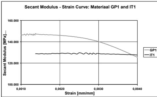
Fig. 6. Calculating the slope from lines from the origin (0,0) to each point of the bending curve produces a diagram of the secant modulus as a function of strain. Material I shows a well defined E-modulus, the value for material G will vary with the selected interval of the curve.
