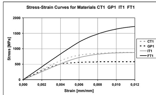
Fig. 11. Stress-Strain curves derived from the Force-Deflection curves from figure 10 with formulas {5} and {6}.
