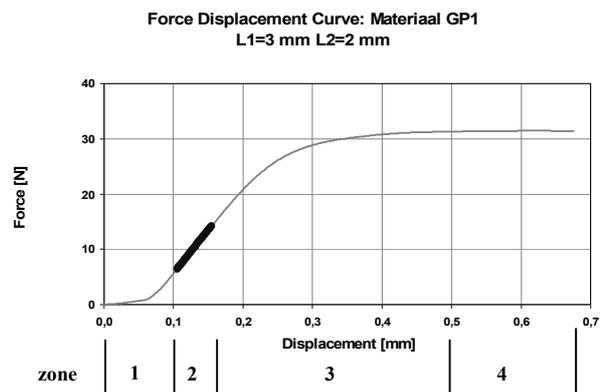
Fig. 5. Example of a measured force-deflection curve, the curve is divided into 4 zones along the horizontal axis.
