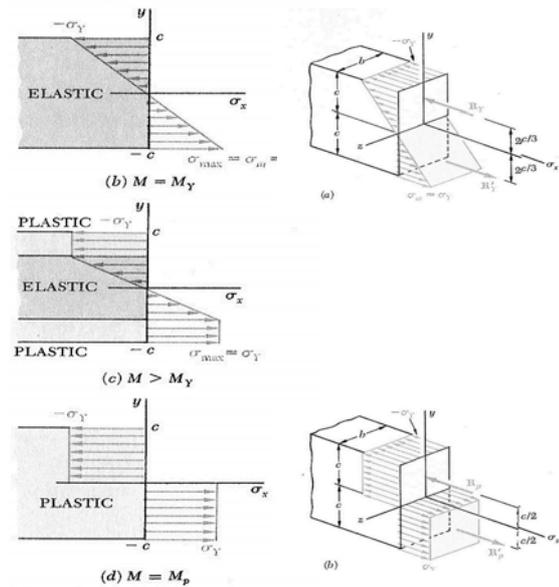
Fig. 7. Stress and strain diagrams from a cantilever beam elastically and plastically deformed. At the top is shown the distribution of elastic stress (zone 2), in the middle the elasto-plastic situation (zone 3) and below the stress during plastic deformation in the cross-section with the highest load.
