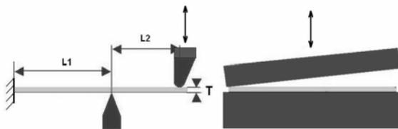
Fig. 8. The proposed set-up for the measurement of the Poisson constant.
