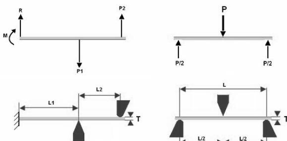
Fig 4. Comparison between mechanical schemes of the PD-test (at the left) and the 3-P bend test (at the right)
