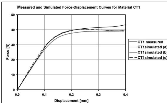
Fig. 13. The measured curve and simulations with bilinear curves (a) and (b) and multilinear curve (c).
