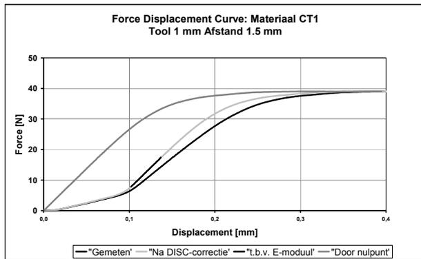
Fig. 9. The measurement curve (black) and illustration of changes to obtain the corrected upper curve.
