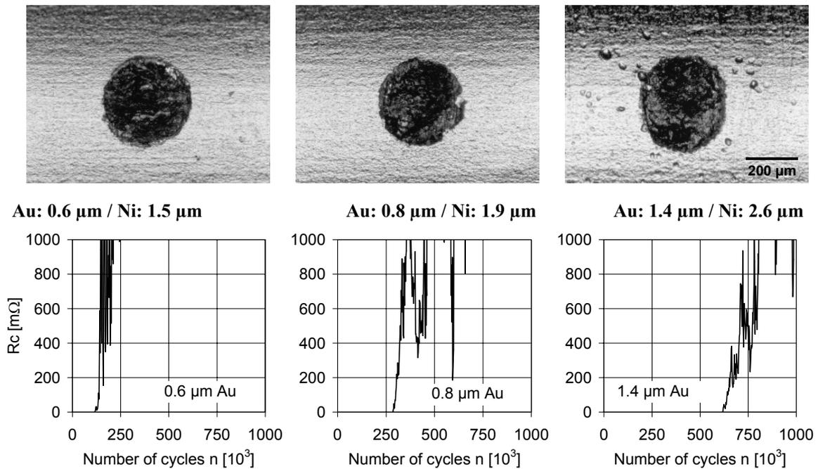
**Fig 11:** Optical micrographs of wear scars on Au coating (with Ni underlayer) of different thickness (top) and evolution of electrical contact resistance, gross slip tests with 20 μm stroke in normal air
