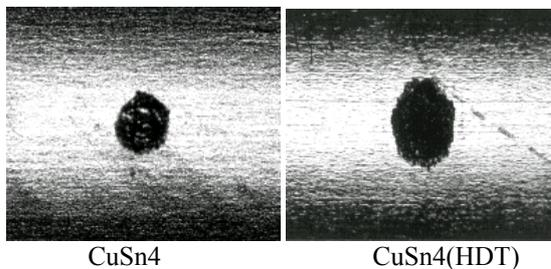
**Fig. 4:** Wear scars on uncoated CuSn4 and on a hdt coated specimen after gross slip fretting
