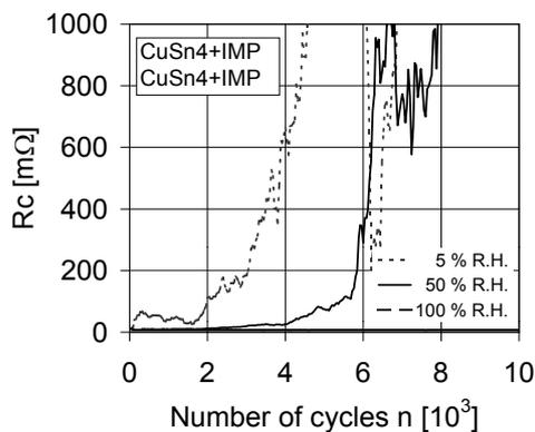
**Fig. 8:** Evolution of electrical resistance in gross slip fretting tests with CuSn4+IMP couple in dry, normal, and moist air
