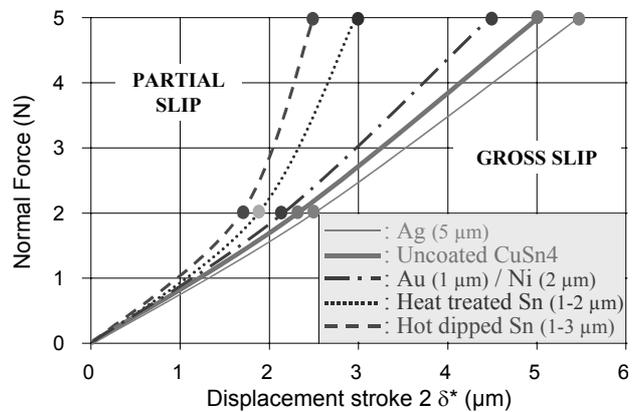
**Fig 5:** Running condition map for different coatings after 10 000 cycles at 10 Hz with 2 N and 5 N load at 45 - 50% R.H.
