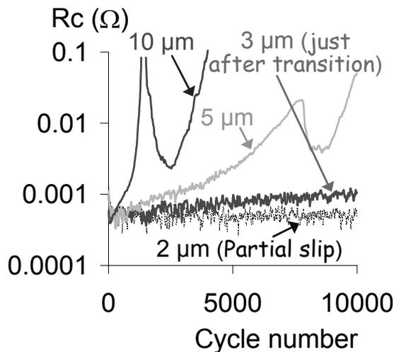
**Fig. 7:** Evolution of electrical resistance in tests with different strokes; hot dip tin coated couple
