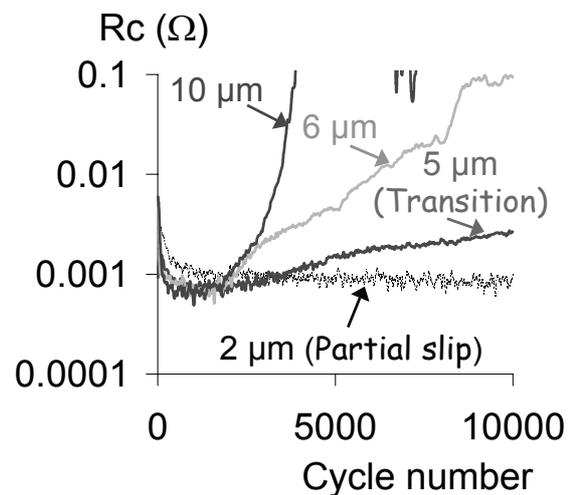
**Fig. 6:** Evolution of electrical resistance in tests with different strokes; uncoated couple
