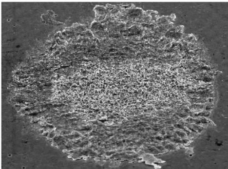
**Fig 2:** Surface appearance of a tin coated contact tested in the partial slip regime
