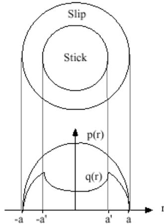
**Fig 1:** Pressure  $p(r)$  and tangential force  $q(r)$  distributions of an elastic fretting contact for a sphere on flat under partial slip conditions
