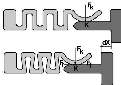
**Fig 12:** Scheme of anti-fretting spring design
