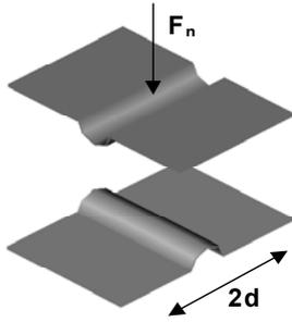
**Fig 3:** Specimen arrangement for "crossed cylinders" [3]
