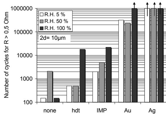
**Fig 9:** Influence of relative humidity (R.H.) on the "life time" of different coatings
