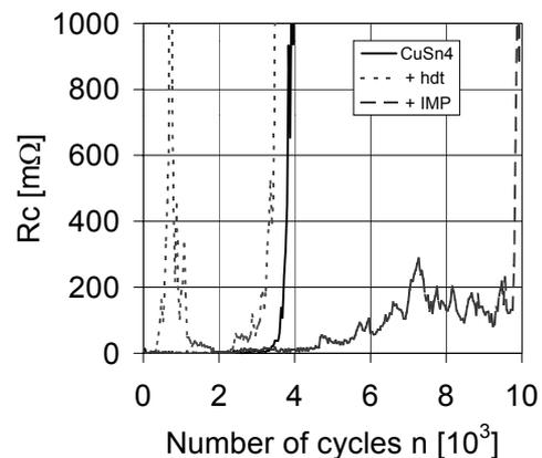
**Fig. 10:** Evolution of electrical contact resistance in gross slip fretting tests with couples of CuSn4, CuSn4+HDT and CuSn4+IMP in normal air,  $2d = 20 \mu\text{m}$ , frequency 10 Hz
